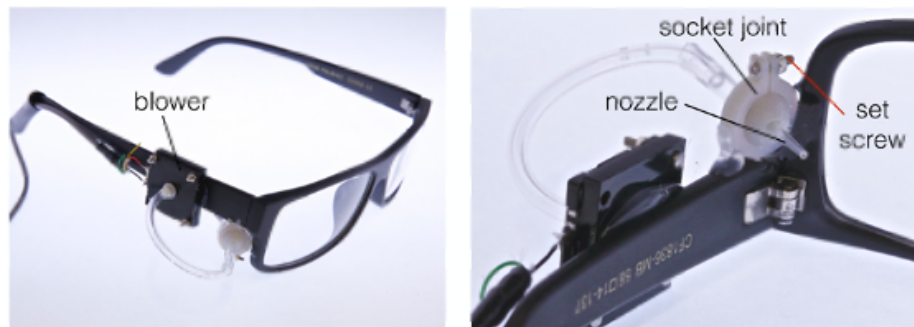
Figure 2.8: Glasses with an air puff construction added to the frame (image taken from [7], © 2017 Dementyev and Holz)
