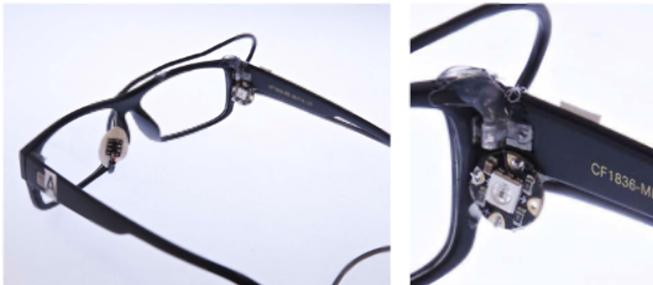
Figure 2.6: Glasses with an LED added to the frame (image taken from [7], © 2017 Dementyev and Holz)
