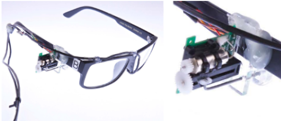
Figure 2.7: Glasses with a servomotor added to the frame to produce taps (image taken from [7], © 2017 Dementyev and Holz)
