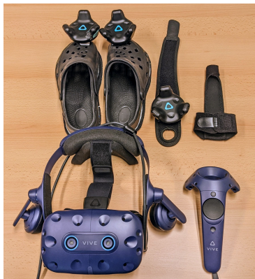
(b) All the equipment worn by a participant during the experiment. This includes a tracked pair of shoes (top left), a tracked fabric and a finger splint (top right), the HTC Vive Pro HMD (bottom left), and an HTC Vive controller (bottom right).
