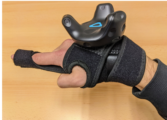
(c) Finger splint and fabric attached to the right hand using a Velcro fastener. The hand is tracked by an HTC Vive tracker that is mounted on the fabric.
