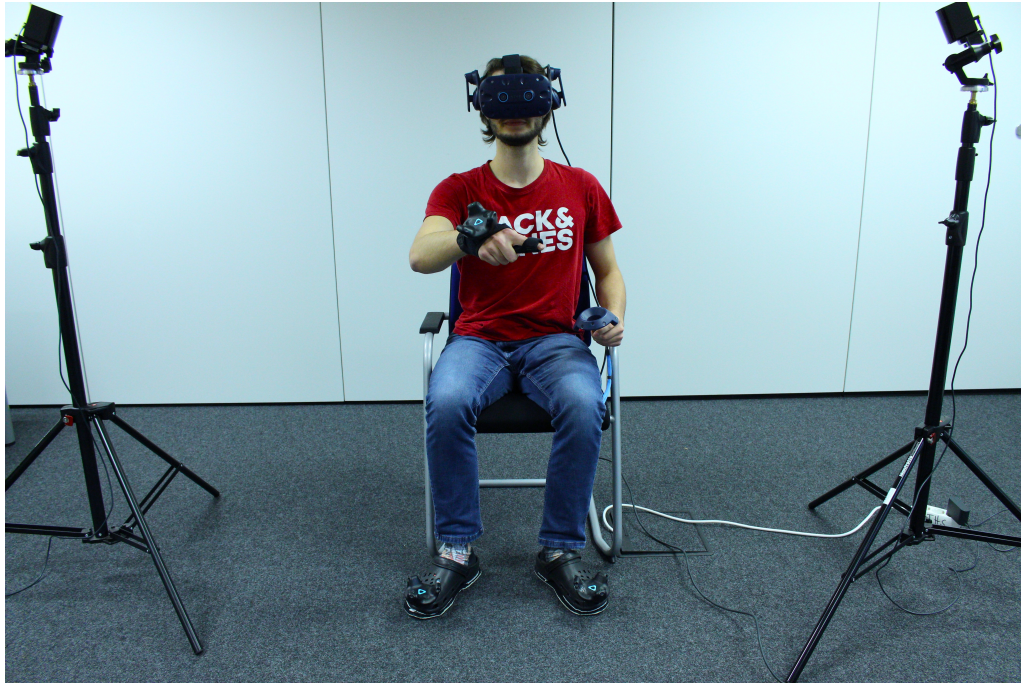
(a) Demonstration of the experiment set-up. The participant is wearing each piece of equipment and is tracked by two HTC base stations.
