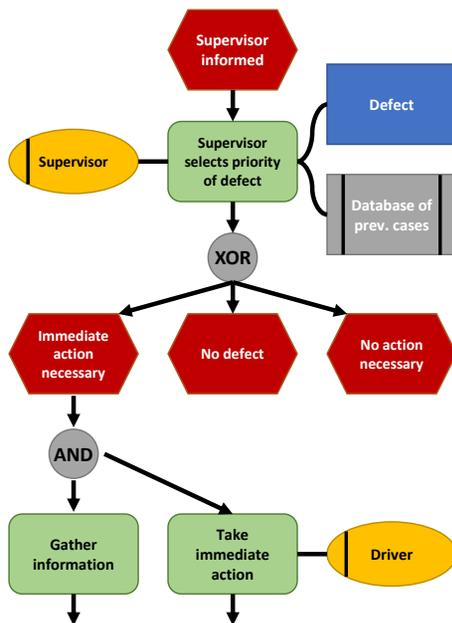
Figure 3: 2D representation of an EPC.
