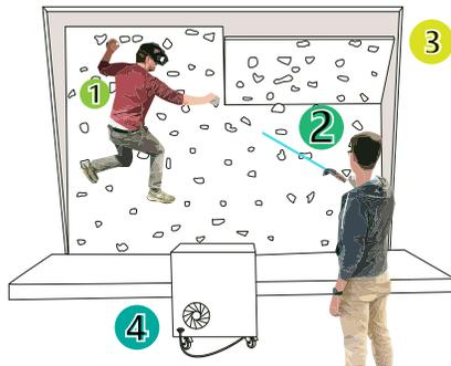
**Figure 3: Our bystander interface (from [13]): The VR user (1) climbs in SR wearing an HMD. An active spectator (2) observes the climber and suggests a hold by pointing into the VE with an HTC Vive controller. Meanwhile, the physical wall (3) is transformed into a spatial augmented reality experience as a projector unit (4) projects the SR onto the physical environment.**
