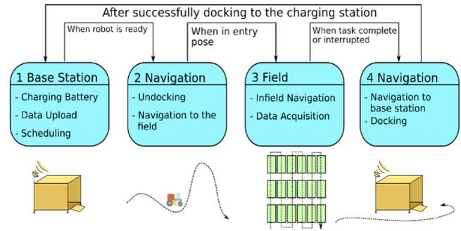
Figure 2: General operation concept of the Valdemar robot.
