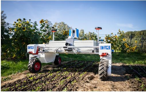
Figure 1: The Valdemar robot equipped with multi-modal sensors for data capture from multiple viewpoints.
