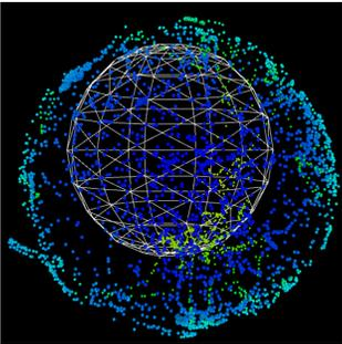
**Figure 2:** Matlab visualization of the 3-axis compass deviation table created with the AHRS firmware
