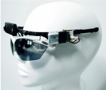
**Figure 1:** Eye tracking prototype extended with sunglasses and a wireless inertial measurement unit to detect the head orientation.
