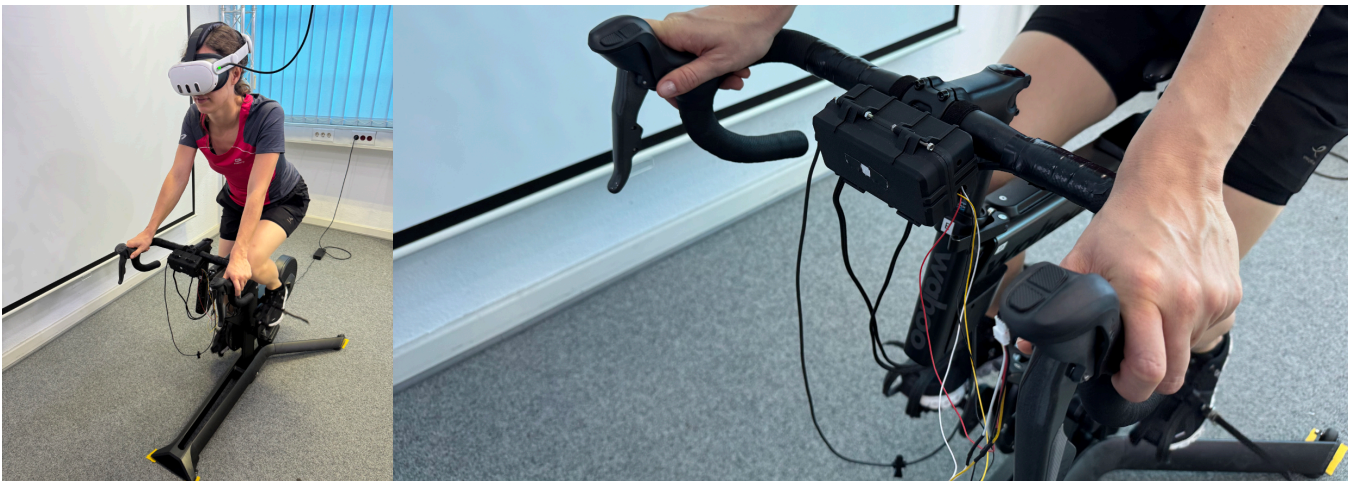
Figure 3: Study setup and buttons. Left: Experimental setup with a participant on the Wahoo KickR Bike wearing a VR headset. Right: Close-up of the handlebar with participants' thumbs placed on the buttons for deciding the 1AFC with "up" or "down". Additionally, a box with an ESP32 microcontroller is attached to the handlebar.
