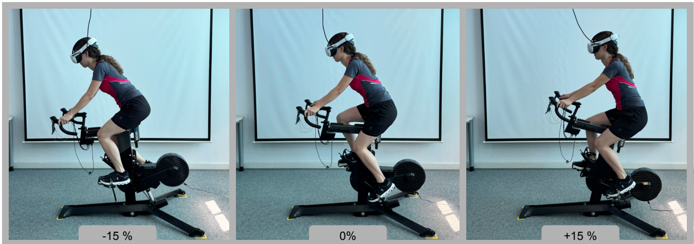
Figure 2: Participant wearing a VR headset experiences real inclinations ranging from -15% to +15% in increments of 5%.
