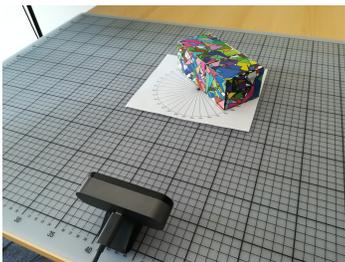
**Figure 5:** Setup for evaluating tracking robustness against perspective distortions, where the same blocks at the same distance are rotated step-wise by 10 degrees between -70 and +70 degrees.
