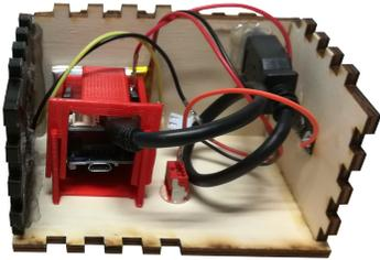
**Figure 2:** Hardware inside the tangibles. For the microprocessor, the Wemos D1 Mini, which includes a WiFi module, is used. Each block contains a battery shield, a lithium-ion polymer rechargeable battery, and a USB charging cable.
