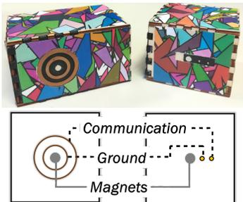
**Figure 3:** For spatial tracking, the tangibles are augmented with fiducial markers (top). Integrated magnets enable easy connections, resulting in contact between the integrated conductive elements (sketched below).
