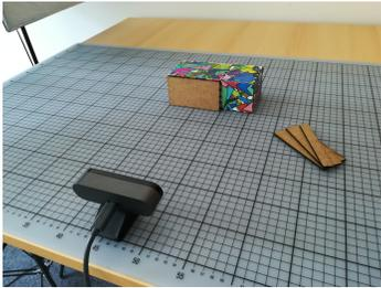
**Figure 4:** Setup for evaluation of tracking robustness against occlusions. One of two connected blocks is occluded using four different laser-cut wooden rectangles of width 10cm and heights corresponding to 25, 50, 75, and 100% occlusion.
