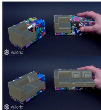
**Figure 1:** A system purely based on marker tracking (top) cannot augment blocks, which are occluded or perspectively distorted. The approach combining marker tracking and embedded computation (bottom) overlays both compositions correctly.
