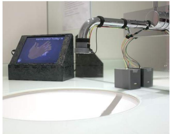
Figure 1. Our system during the in-the-wild study: A 3D-printed measuring unit which can be mounted on the tap and a gameful mobile application. The measuring unit detects whether water is running and whether hands are present or not and sends this information to the mobile application.
