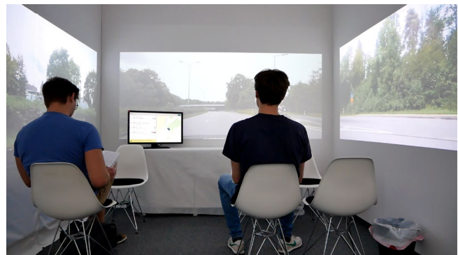
Figure 1. Immersive video-based autonomous vehicle simulator with a 26-inch passenger information display.
