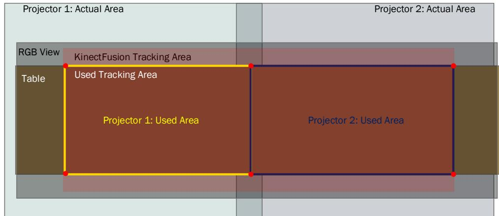
Figure 4.18: The different spaces used for calibrating the projectors.
