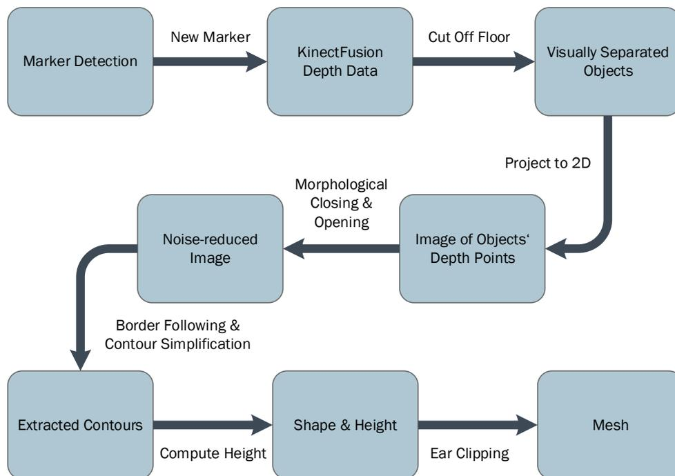
Figure 4.3: Overview of the object recognition process.
