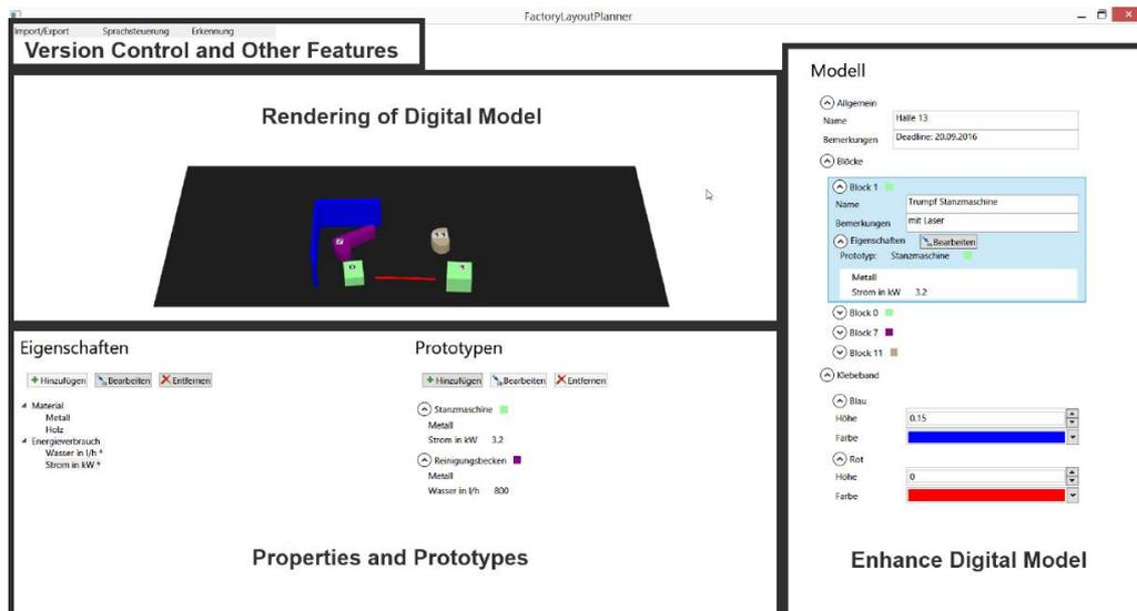
Figure 3.6: DEPlaTa’s Graphical User Interface with overlays for the different sections.
