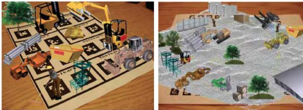
Figure 2.8: A tangible AR system for construction site planning called AR Planner [56].
