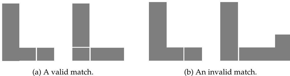
Figure 4.16: Matches between cached and currently found contours.
