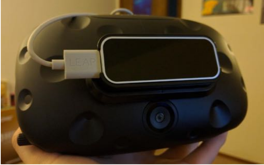
Figure 5.1: The used Output (HTC VIVE) and Input (Leap Motion) Setup 1
