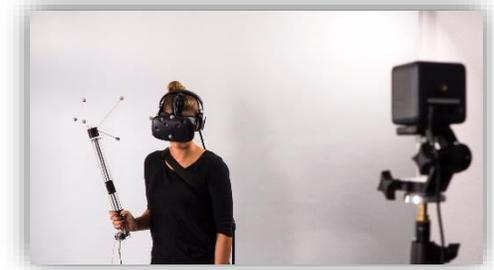
By shifting an internal mass, *Shifty* **can change the weight and inertia** felt by the user during VR interaction. When combined with corresponding visualizations in VR, this haptic effect can **convey the feeling of virtual object weights, shapes, and materials**.
