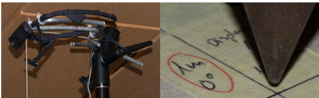
Figure 31: [Left] Pupil Pro eye tracker mounted on a tripod. [Right] Plumb bob attached to the tripod for precise positioning at predefined locations in front of the display.
