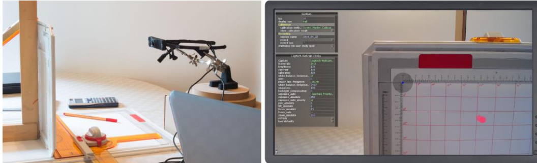
Figure 13: Apparatus to investigate FOV of the Pupil tracker's scene camera (left) and the corresponding camera still frame (right).
