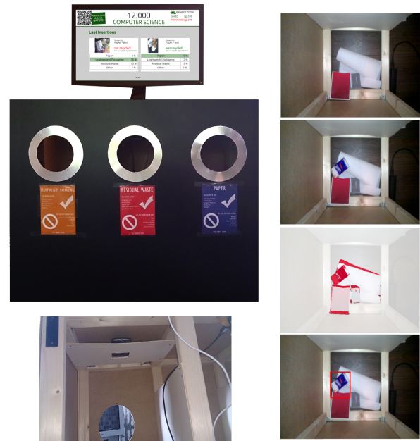
Figure 5. Left: Exterior/interior of the prototype. Right: Steps of extraction algorithm: (From top to bottom) Before insertions, after insertions, recognized differences, red rectangle showing extracted picture.
